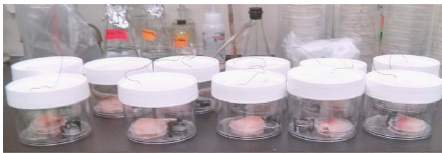
Fig. 3. Samples of tilapia tissue kept at 24\text{ }^\circ\text{C} for microbial analysis. Each jar contains a 25 g tissue sample of fish and a hydrogel coated pH-sensitive electrode pair with wired connection to a voltmeter.
